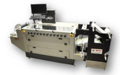
Designed for roll-to-roll printing of license plate reflective sheeting up to 12.125" wide, the DigiTag 1650™ Printing System prints your license plate graphics in 4-color process plus 2 spot colors, or up to 6 spot colors, at a maximum resolution of 1600 x 400 dpi. With a highly productive speed up to 905 ft./hour,a robust processor and powerful software, the DigiTag 1650 can efficiently print variable license plate information on-the-fly.
